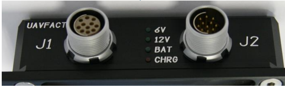
Figure 11 Input, Output connectors and status LEDs
